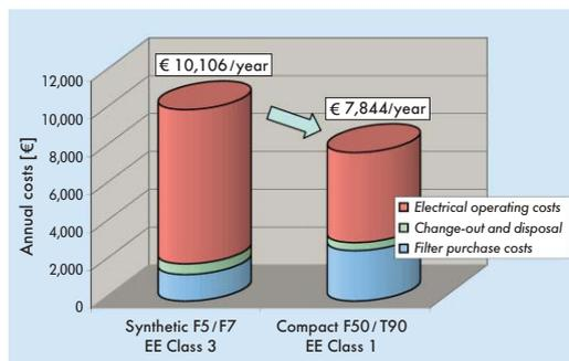
Example: 100,000 m<sup>3</sup>/h system, two filter stages, F5/F7
