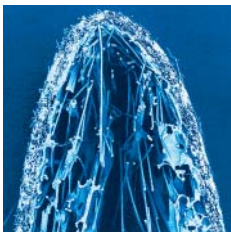
Drainage nonwoven, SEM photo
