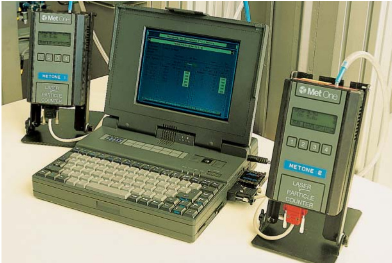
Particle counter for measuring the dust concentration on-site
