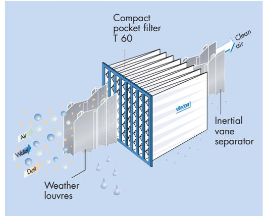
Viledon T 60 pocket filter in a vane-coalescer-vane system
