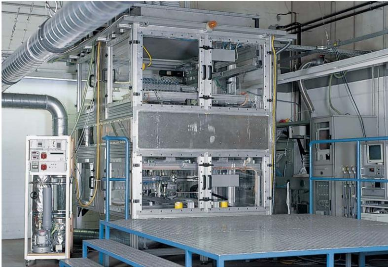
Multi-scanner for HEPA and ULPA filters
