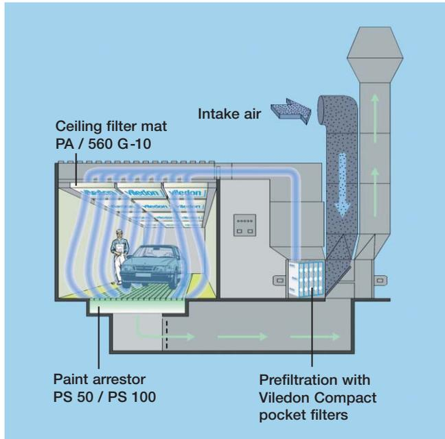
Fig. 3 Schematic depiction of a repair cabin
