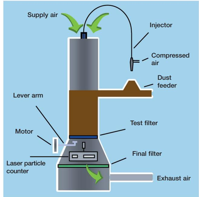
Fig. 7 Filter test rig for the migration test
