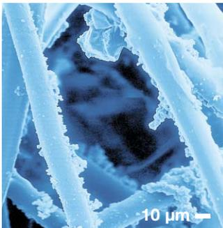
Fig. 6 Fibers with an actively adhesive finish, showing the retained particles
